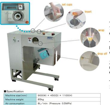
The gerbera cup machine can save you up to 70% in labour compared with putting on the cups by hand.
